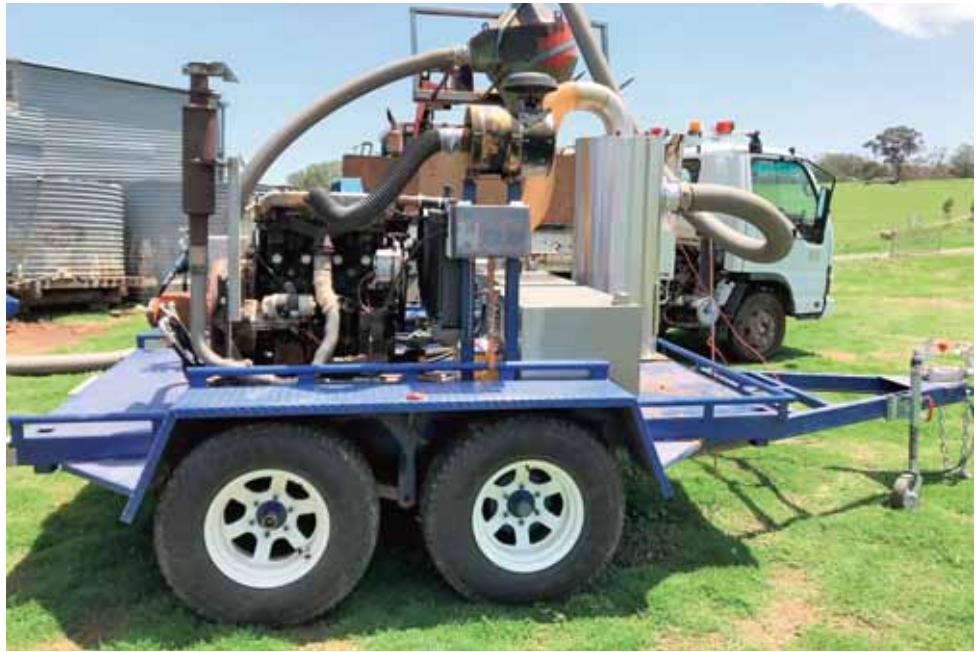
A mobile solution to a common on-farm problem - a trailer mounted vacuum
